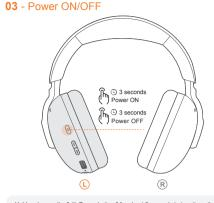
Hold and press the " (I) Power button " for about 3 seconds to turn it on, the Mode Hold and press the " (I) Power button " for about 3 seconds to turn it off, the Mode Indicator off.
